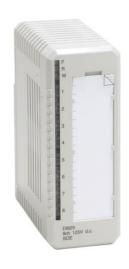
The DI825 is an 8 channel 125 V d.c. digital input module for the S800 I/O. The input range is 71 - 150 V and the input current is 3.0 mA at 125 V. The inputs are individually isolated.
